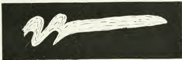
Fig. 38—Fragment of schist in sulphides, sixth level, Garson mine, Sudbury area, Ontario. The majority of rock fragments in the ore at Garson mine are schists or schistose rocks. Width of face 15 inches.
